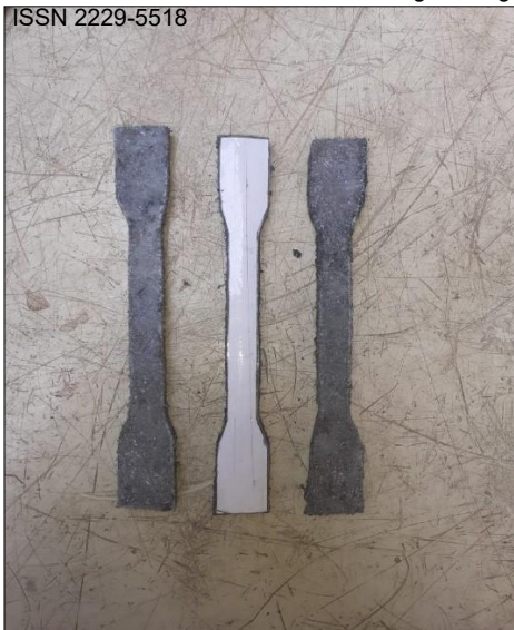
Fig 1. Tensile Test Specimens
